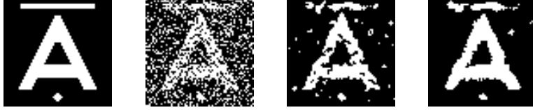
Figure 5.1: The 64 \times 64 binary image of an "A" by Greig et al. (1989) (a), the same image corrupted with salt and pepper noise with parameter q = 0.25 (b), the estimated true image using the model described in Section 5.1 with n = 3 (c), and the estimate using the same model, but with n = 5 (d).
